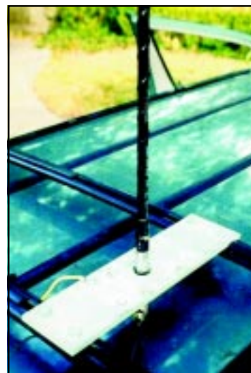
A close-up view of my Hamstick mobile antenna mount using the Lumina’s luggage rack.
